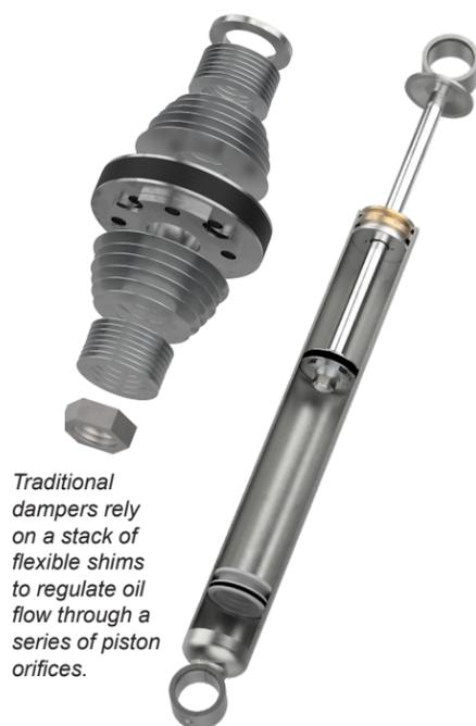
Traditional dampers rely on a stack of flexible shims to regulate oil flow through a series of piston orifices.
